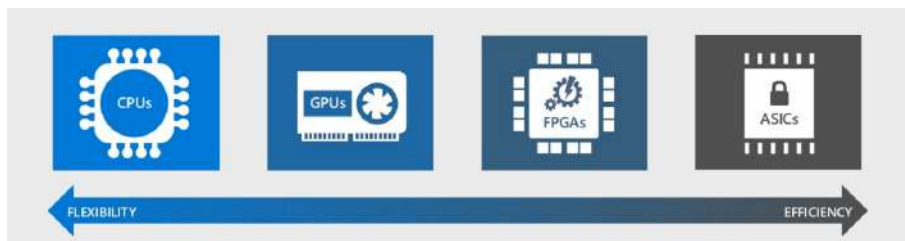
Figure 7: Flexibility vs. Efficiency for different computing platforms. Source Microsoft.
